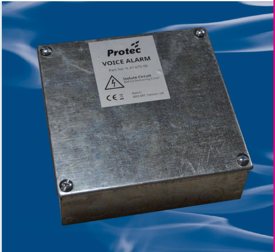
This square galvanised, metal enclosure is a wall mounted Voice Alarm junction box for Voice Alarm loudspeakers and tenants extension circuits. It comes complete with ceramic terminal blocks.
