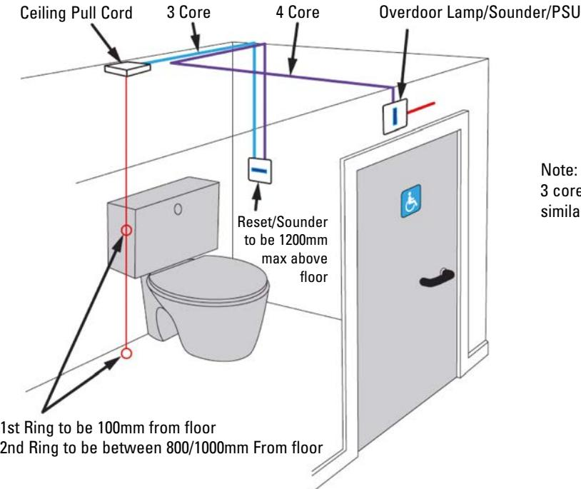
Note: CAT 5 STP type cable should be used for the 3 core and 4 core interlink wiring. Twin and Earth or similar rigid type cables should never be used.
