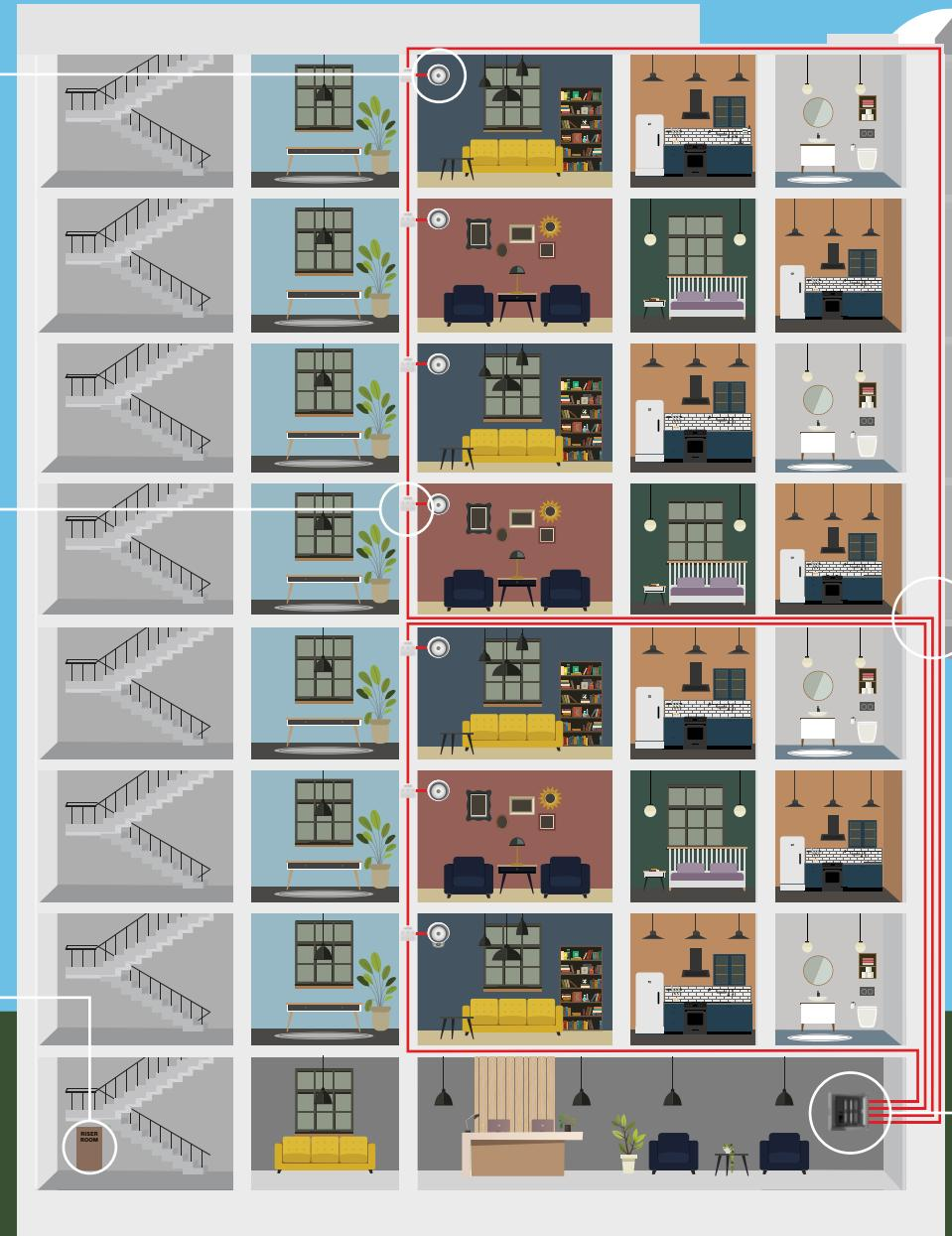
The EvacPro is wired in a loop configuration to provide redundancy in the event of a fault. Enhanced fire rated cable is used throughout.
