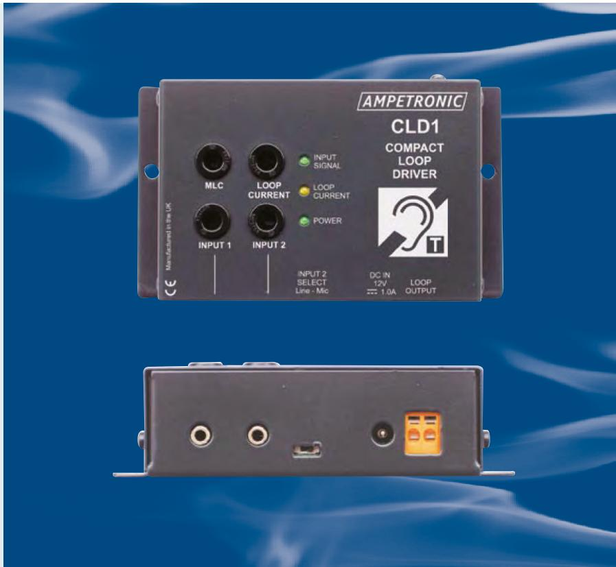
The CLD1 Compact Loop Driver is designed for counter systems and small area perimeter loop systems. Measuring only 128 x 74 x 35mm and with an output current of 2.4A RMS, the CLD1 is the smallest and highest performance amplifier in its class. Designed and built to Protec's high standards of reliability, and backed with a 5 year warranty, the CLD1 offers certainty of performance and the lowest lifetime cost available.
