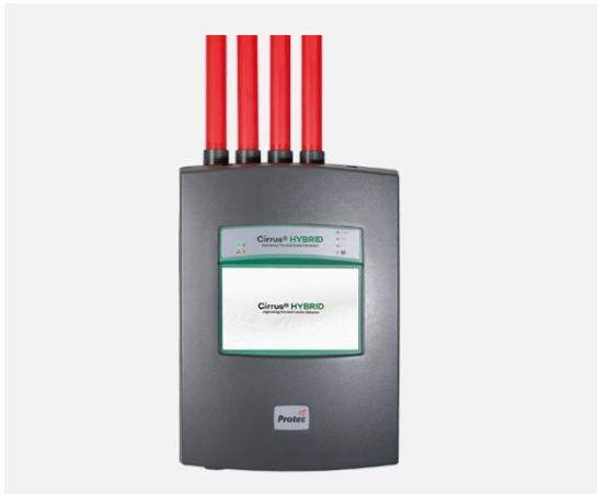
The Cirrus HYBRID aspirating detector combines Scatter and Cloud Chamber detection technologies into one unit. With the ability to cover up to four pipes, this dual technology approach provides excellent sensitivity for detecting fire and smoke while significantly reducing false alarms.
