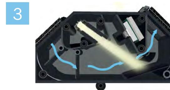
A beam of light is transmitted from the emitter.
