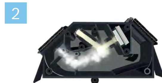
Air enters the aspirating unit and is directed into the Scatter Chamber Detector modules for optical analysis of visible smoke particles.
