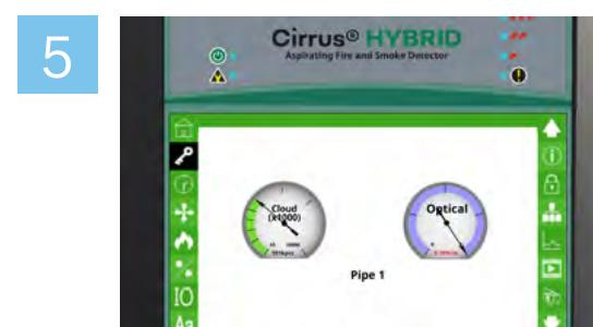
AI technology combines the smoke signals from the optic sensors and the cloud chamber sensor, enabling only true alarms to be verified.
