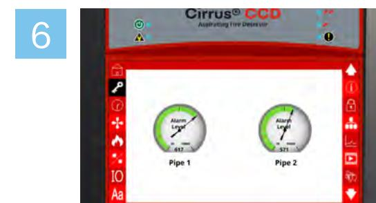
An alarm condition is initiated when combustion particles are greater than the programmed fire condition thresholds.
