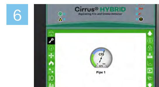
A fire condition is initiated if the fire/smoke particles are greater than the preset fire alarm thresholds.
