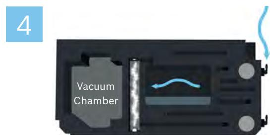
The result is the instant formation of water droplets on fire particles within the sampled air, thereby forming a cloud in the chamber.
