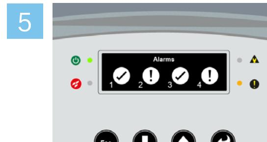
An alarm condition is initiated when smoke particles are greater than the programmed smoke alarm thresholds.
