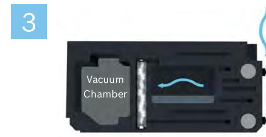
The air is drawn through the cloud chamber into a humid vacuum. The vacuum is removed. Moisture in the chamber condenses onto the fire particles, creating a cloud.
