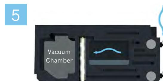
The cloud density is measured in the cloud chamber sensor.
