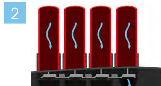
Air enters the aspirating unit and is directed into the Scatter Chamber Detectors.
