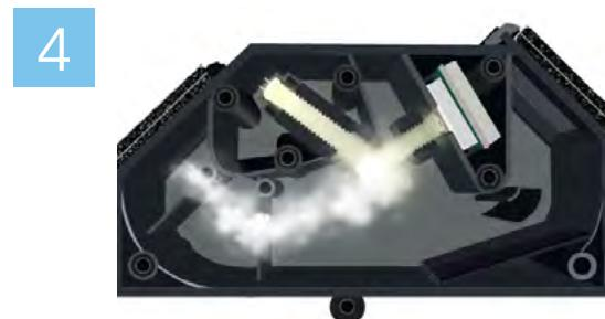
This beam is scattered onto a light receiver when visible smoke particles are present.
