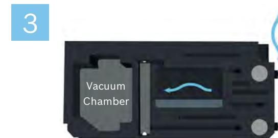
Pressure and temperature changes are initiated within the Cloud Chamber.
