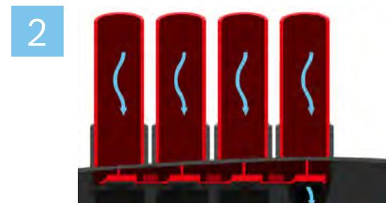
Air enters the aspirating unit and is directed into the Cloud Chamber Detector.
