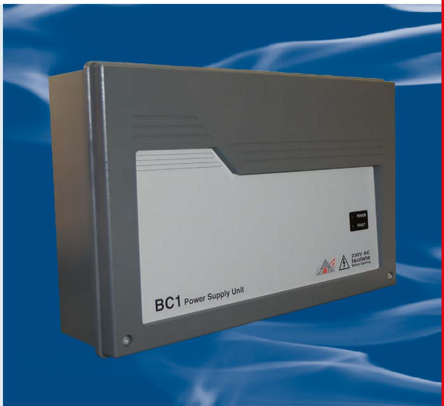
The Protec 9000/BC1 is a 24V dc 1A intelligent power supply and battery charger designed to be used in conjunction with two 12V 3.3Ah Sealed Lead Acid batteries. The charger continuously monitors various critical levels and gives a fault warning if any of the levels are out of specified limits.
