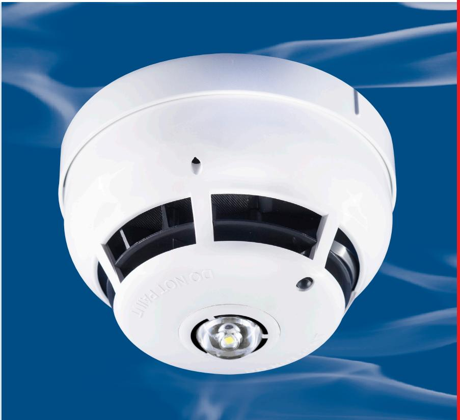
The Protec Algo-Tec™ 6000*PLUS* sensor range have been developed to incorporate advanced fire sensing technology, electronic sounders, high intensity LED visual alarm devices (VAD) and speech enhanced talking sounder capability, all integrated within the sensor head and powered from the loop.
