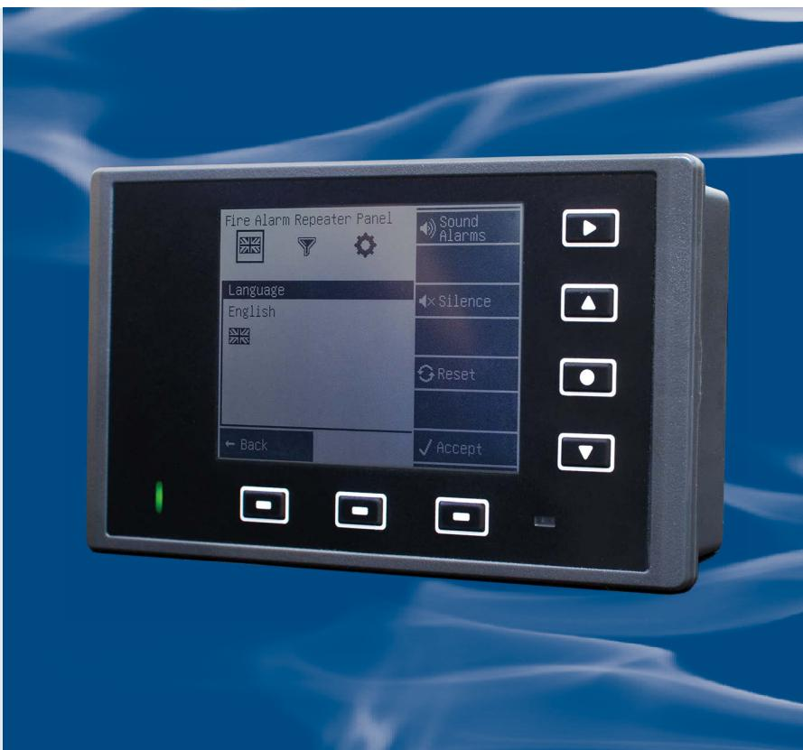
The 6000PLUS/REPEATER can be connected directly to the local Algo-Tec™ digital addressable data loop and takes up just one address. Events from the main panel are displayed on the repeater's large LCD display, providing system indication of any loop connected location on site. The low power consumption allows numerous repeat devices to be fitted, greatly increasing system visibility.
