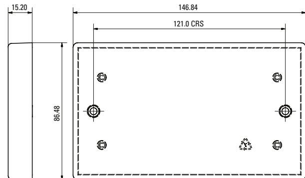
Backbox Requirements - Surface or flush double gang pattress box minimum of 25mm deep.
