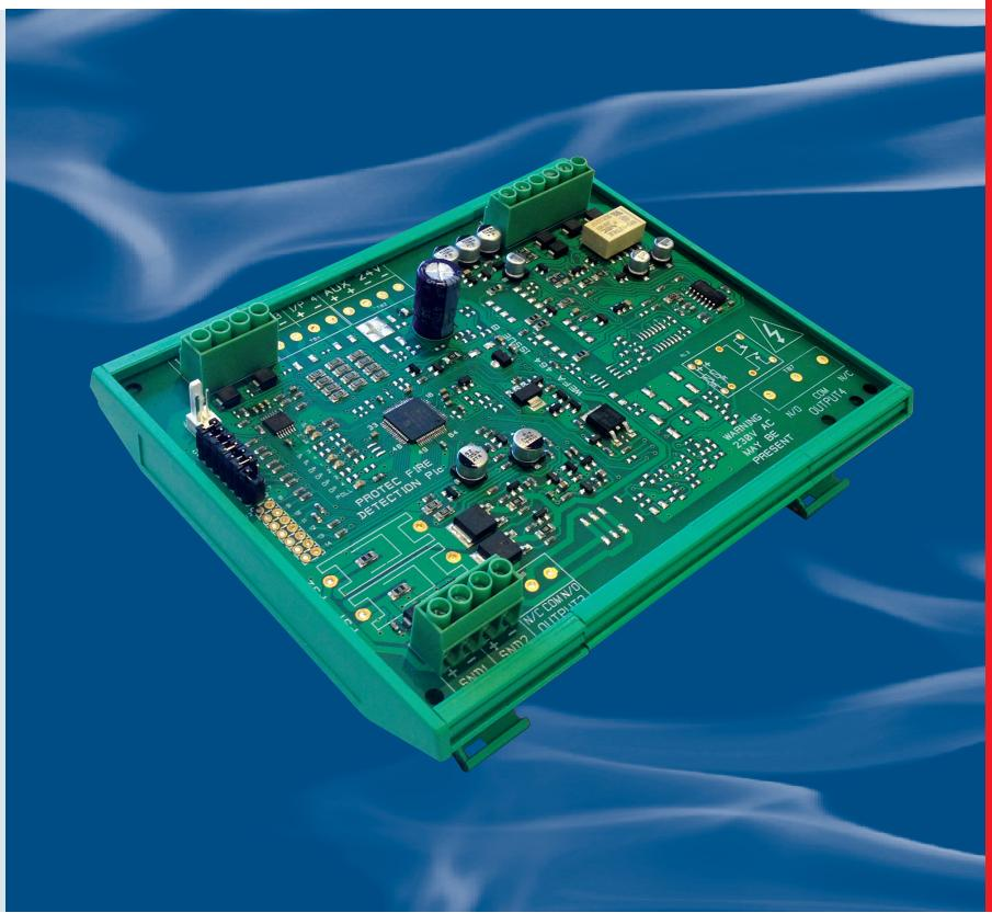
The Protec 2 way loop zone alarm interface is a loop powered input / output device providing 2 local zones of conventional detectors and 2 local monitored alarm outputs.
