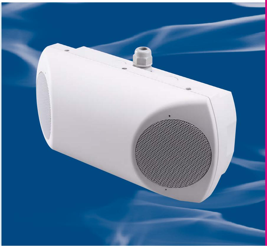
This bi-directional cabinet loudspeaker is constructed from LSOH plastic and can be installed on solid ceilings or walls. Supplied with dual gland entries, which give the installer the option of loop in loop out termination thus avoiding the need for a separate junction box, this cabinet is both robust and aesthetically pleasing. Although our standard finish is White, RAL9016, alternative finishes are available upon request.
