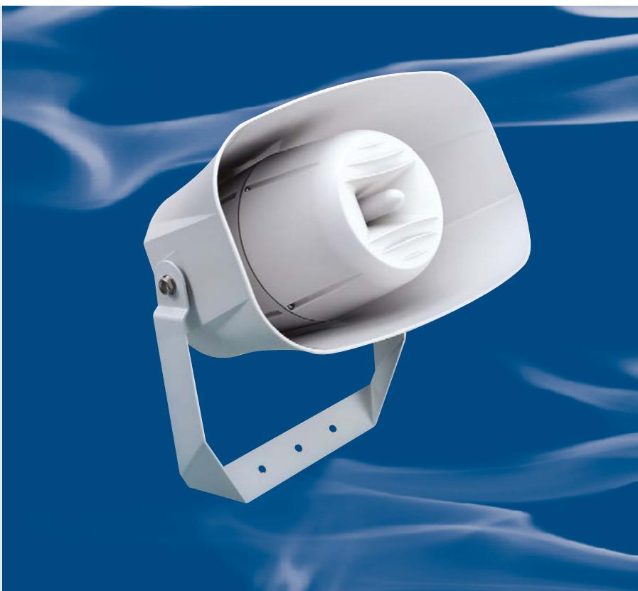
This weatherproof plastic horn loudspeaker combines a re-entrant horn with a high frequency unit and has been developed for clear speech and quality background music reproduction. The unit is rated at 30 watts and has two drive units one for low end frequencies and one for high, producing a unique sound quality.
